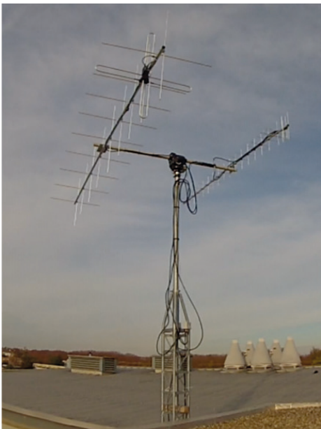
VHF antenna (2x10 elements) and UHF antenna (2x17 elements) of F4KLD ( https://youtu.be/2lGayGdK42E )
